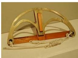
This is a Rudder Yoke. Steering ropes or lines run from holes in the ends of the yoke arms allowing steering from nearly anywhere in the boat. It allowed the boat's helmsman to sit way aft while looking forward and steering the boat by pulling on the tiller lines.
