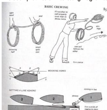
Fig. 35. Careful coiling is the secret when throwing a heaving line. Divide the coil as shown and remember to aim high. There's a knack to throwing a line and it needs practice.
